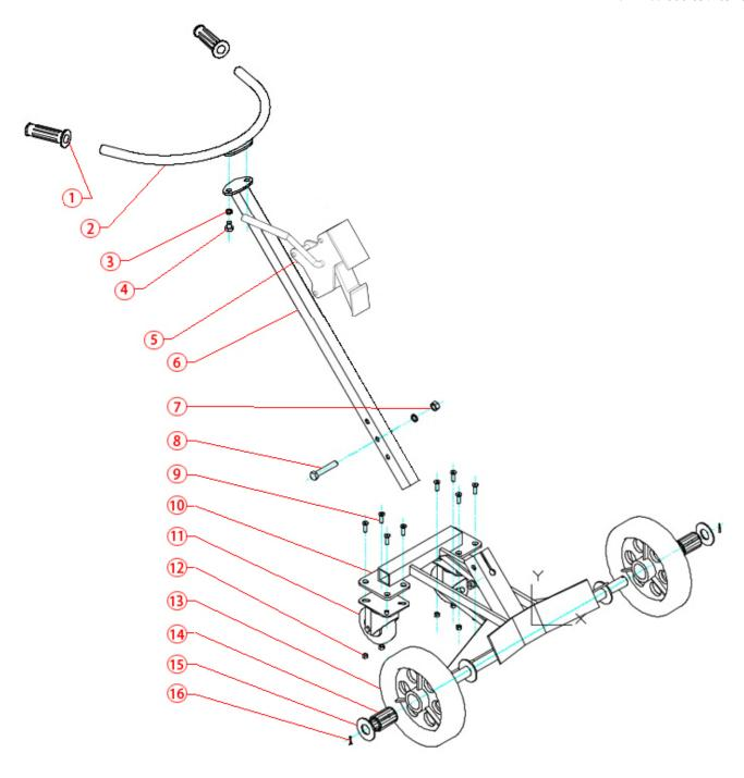
SCHEMATIC for 10HT-PNC DRUM HAND TRUCK
